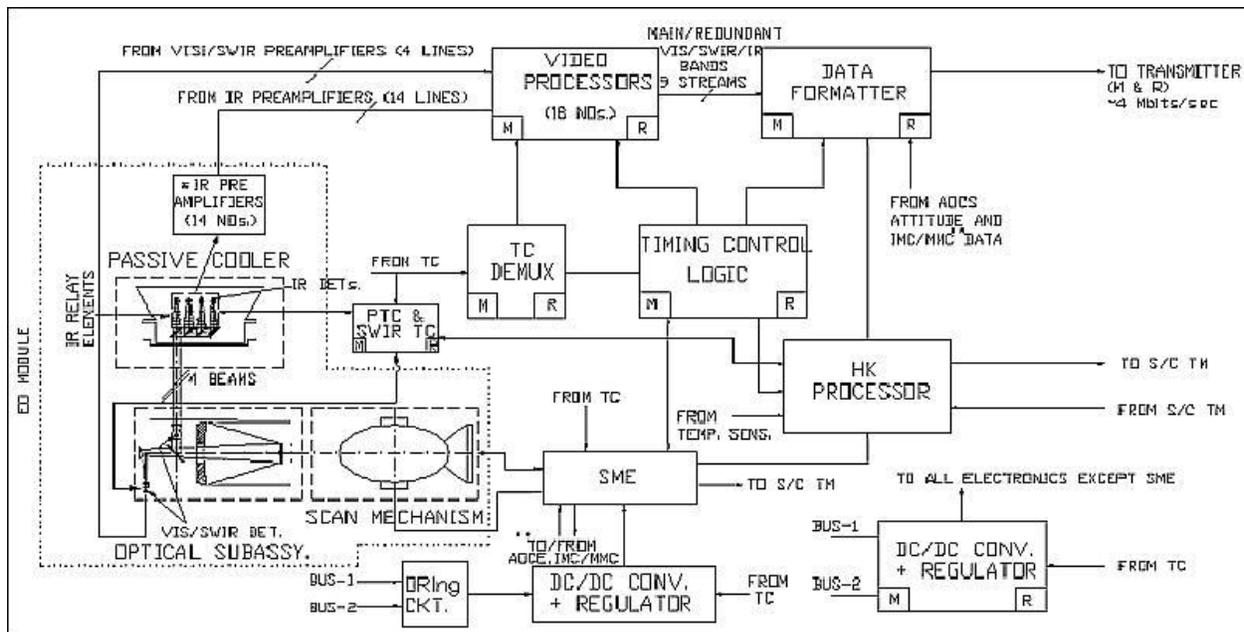
Figure 7: Block schematic of INSAT-3D Imager
