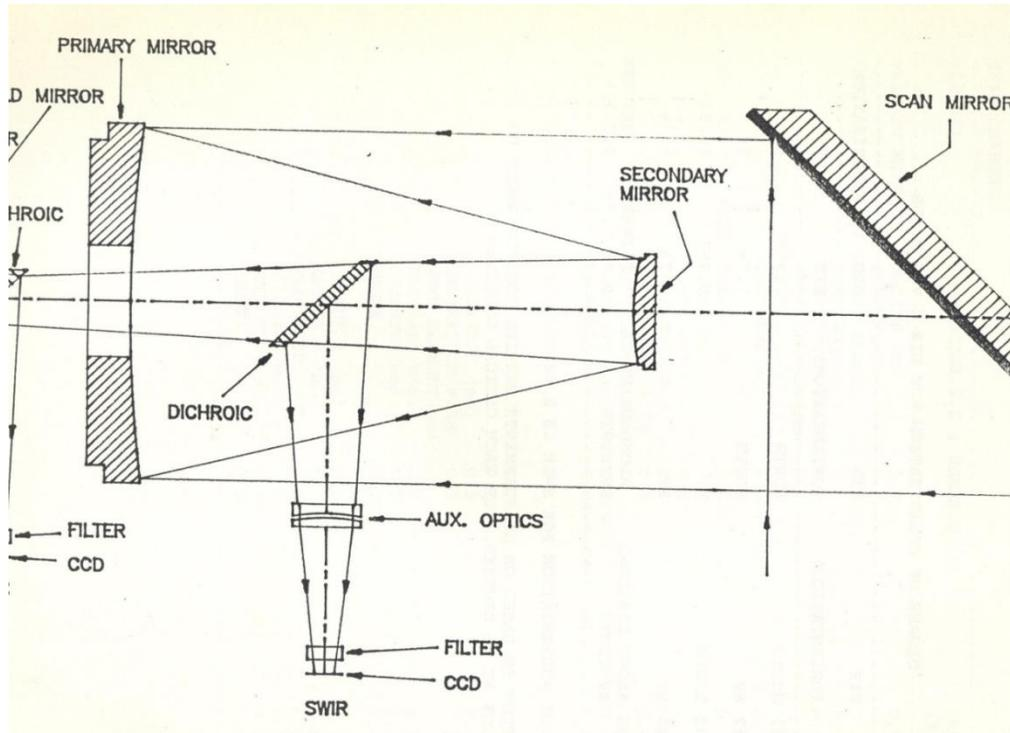
Fig.4: Optics schematic of INSAT-2E CCD Payload
