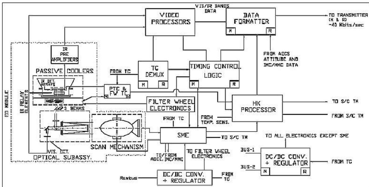
Figure 10: Block schematic of INSAT-3D IR Sounder
