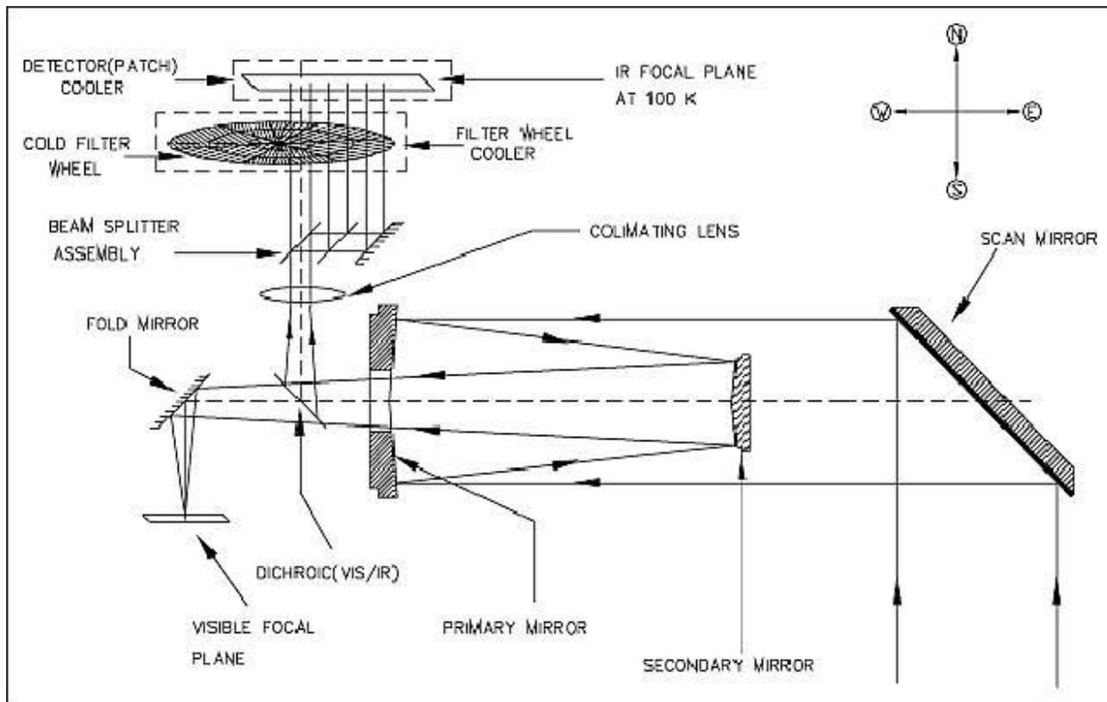
Figure 12: INSAT-3D Sounder Optics Schematic
